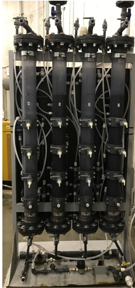
Figures 1 & 2: Photos of front and rear of pilot unit showing 4 columns, flow meters, and interconnecting piping.
