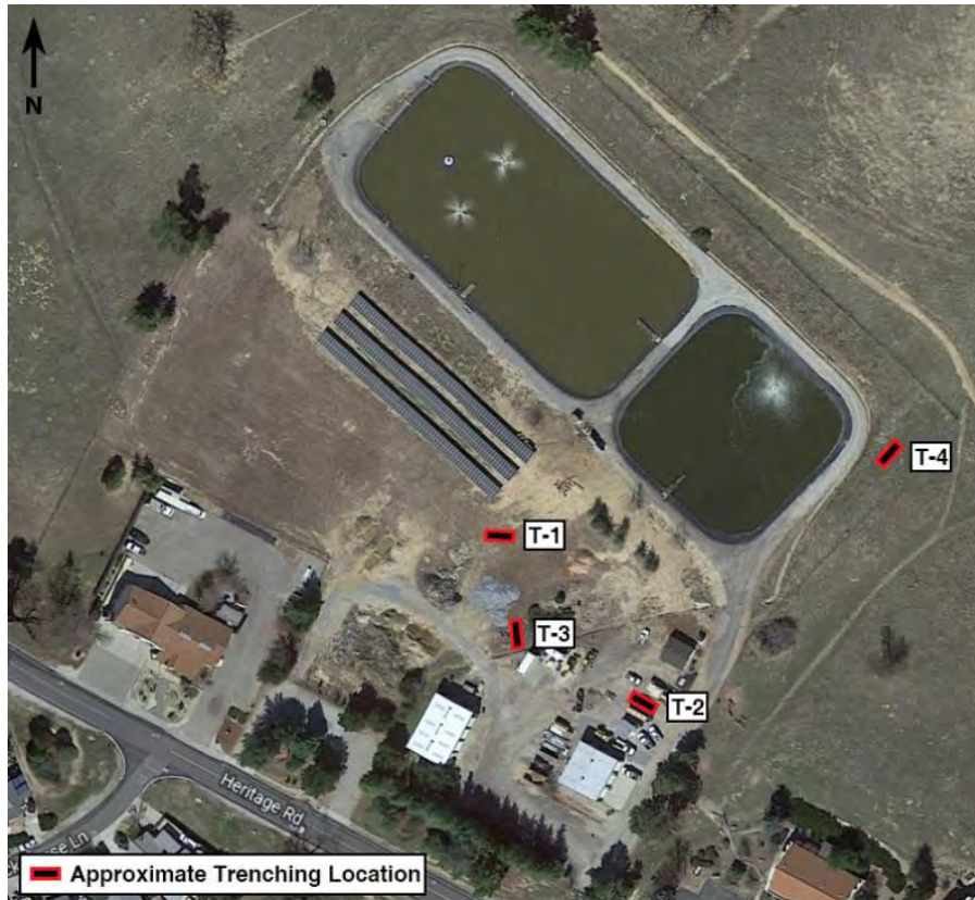
Figure 25 Geotechnical Site Investigation Trenching Locations
